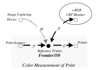
Figure 2. Color transform between devices
