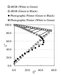
Figure 6. Result of gamut mapping (method B) between sRGB and laser photographic printer plotted in L\*-C\* plane at Hab=180
