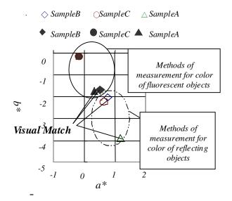
Figure 3. Plots of colorimetric values of photographic color paper by two different measurement methods, Sample A and B match visually
