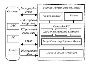
Figure 1. Fujifilm's digital imaging services
