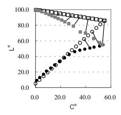
Figure 5. Result of gamut mapping (method A) between sRGB and laser photographic printer plotted in L\*-C\* plane at Hab=180
